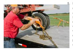
Inspect tie downs for wear and damage. CVSA's North American Standard Out-of-Service Criteria includes the tie down defect tables for chain, wire rope, cordage, synthetic webbing, steel strapping, fittings or attachments and anchor points. If worn out, tie downs should be discarded.
