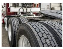
some road temperatures can reach almost 200° F, the heat problems caused by under inflation are more extreme. Tires that are run under inflated will be more prone to failure in these temperatures. A very famous tire engineer once stated, "Heat is to tires as Kryponite is to Superman"... in other words, it's worst enemy. Taken all together, hot summer temperatures, under inflated tires, heavy loads, and traveling at high speeds (not that this ever happens), and
