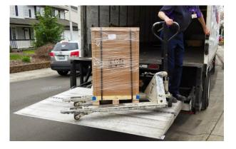
that a liftgate will drain a battery after 7-10 cycles, most stops do not require that level of use. Additionally, all our Idealease units with liftgates have low voltage protection. So, the driver can be confident that if the liftgates goes through multiple cycles and stops, the truck will still start without issue.
