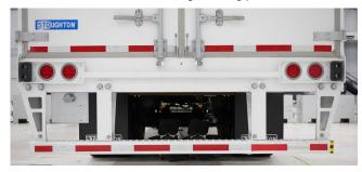
The Federal Motor Carrier Safety Administration has published a final rule to include rear impact guards on the list of items that must be examined as part of the required annual inspection for each commercial motor vehicle. 86 Fed. Reg. 62105 (November 9, 2021).
