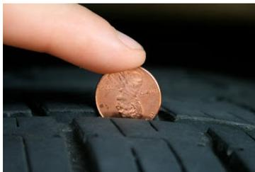
The last tip about measuring tread depth: never measure in the decoupling groove which is found in many steer tire designs to reduce irregular wear. This outside decoupling groove is sometimes known as a PDG groove (Pressure Distribution Groove) and they may be very deep or may be very shallow but it is not the same depth as the major tire grooves.
