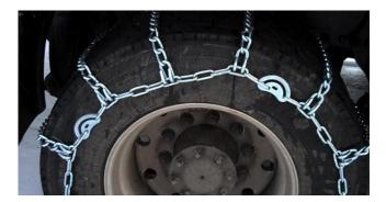
If you are operating in a state that requires chains to be on board, make sure the chains are the correct size, properly secured, clean, undamaged/easily accessible when necessary.
