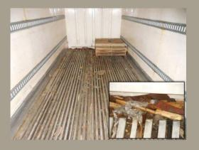
Of all the things that the operator of a refrigerated truck could do to seriously impact the ability to maintain temperature, cleaning the back of the truck is the most significant. At the end of every workday, the driver of the truck should inspect and clean the inside of the truck box. This means making certain there is no paper, cardboard, shrink wrap, or anything else that may cause a restriction of airflow around loaded product.
