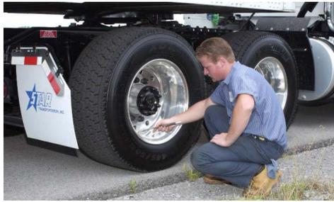
**Prevention:** Pre and Post Trip inspections that identify tires that are getting close to regulation requirements being reported on the daily vehicle inspection report. Drivers need to know how and when to check inflation (with a gauge!) and when it's time for a replacement.
